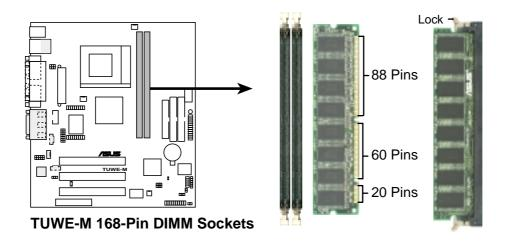
The DIMMs must be 3.3 Volt unbuffered SDRAMs. To determine the DIMM type, check the notches on the DIMMs (see figure below).
